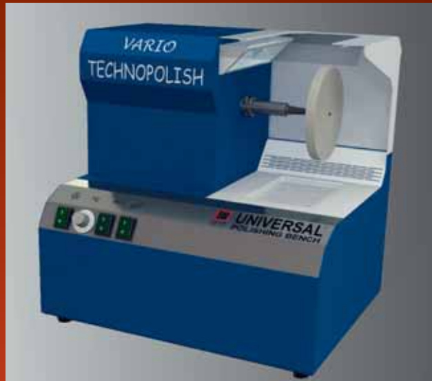
BM 82A (982.82.001) POLISHING BENCH ( Variable Speed Control ) 0,55 kW / 230 V, 50 Hz 300 – 3000 rpm Vacuum 750 m 3 /h
